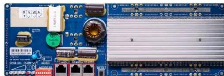
RS485 Communication between battery and inverter Band rate: 9600bps RS485 Interface Communication between parallel packs of BMS and PC Band rate: 9600bps
